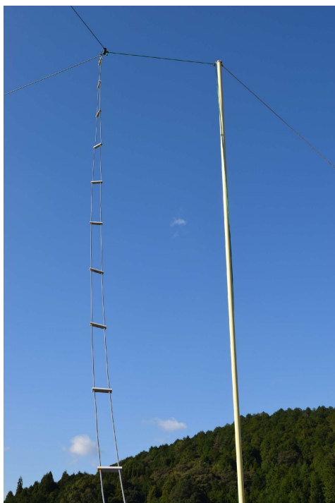
Fig.2: Feeding Method Using a Parallel Feeder
