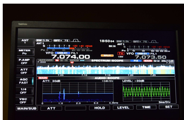
Fig.10: Noise situation of 40mBand 3\lambda Square Loop
